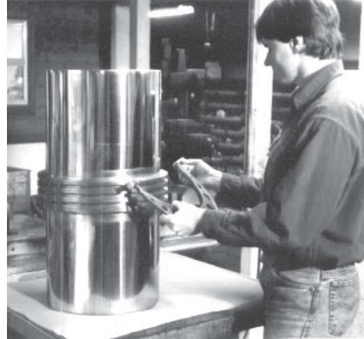
INSPECTION OF A 2016 DRAG CONTROL PISTON AFTER FINAL O.D. POLISHING
